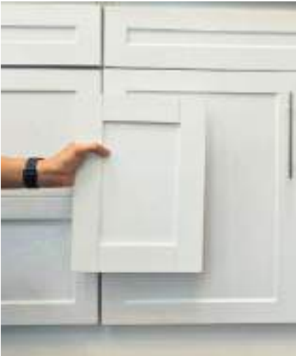
Inspecting Material, Surface & Color Quality Every component is thoroughly inspected for material consistency, surface smoothness, and color uniformity. Any product showing color deviation, surface defect, or material inconsistency is immediately rejected. This ensures that only perfectly matched and high-quality cabinets are approved for delivery.
