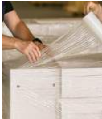
1. Protective wrapping for each cabinet module
