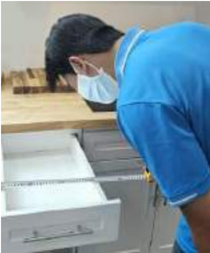
Measuring Cabinet & Drawer Dimensions Each cabinet and drawer is carefully measured and inspected to ensure precise sizing, perfect alignment, and smooth functionality. This process guarantees that every component meets strict quality standards before packaging and shipment.
